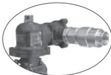
Use packing at the through portion of outside conductor, and cable is used as outside conductor. Connect pressure-proof packing gland to the through portion for significant part 5 screw thread and more. First tighten the gland as strong as possible by locknut, next tighten the pressure-proof packing part and lock the cable.
