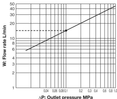
• How to determine the flow rate (Steam, Air)
